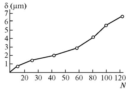
Fig. 4. The relation between the quantity of machining parts and abrasion on tools in vibration cutting ferrous metals with diamond tool.
