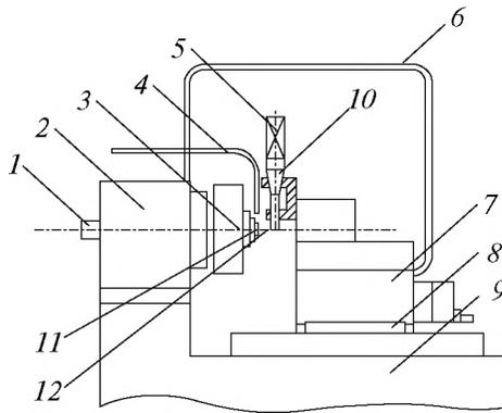
Fig. 1. The experimental schematic of application of carbon dioxide in ultrasonic vibration cutting titanium alloy.
