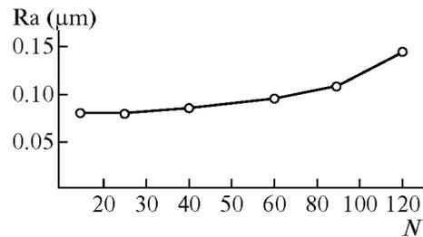
Fig. 5. The relation between the quantity of machining parts and roughness in the system of carbon-saturated vibration cutting ferrous metals with diamond tool.
