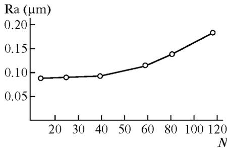
Fig. 3. The relation between the quantity of machining parts and roughness in vibration cutting ferrous metals with diamond tool.
