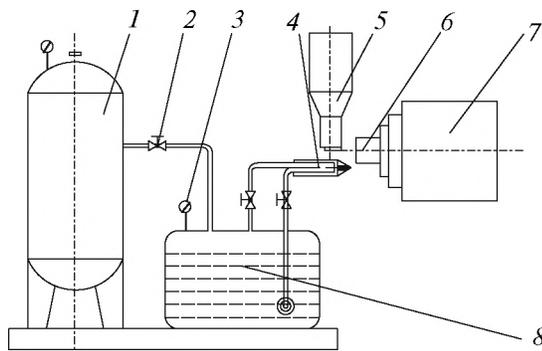
Fig. 2. The diagram for gas-fluid atomization device in cutting experiment.
